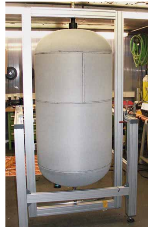
Lined tanks suspended in the testing apparatus for measuring and for helium-based examination.
